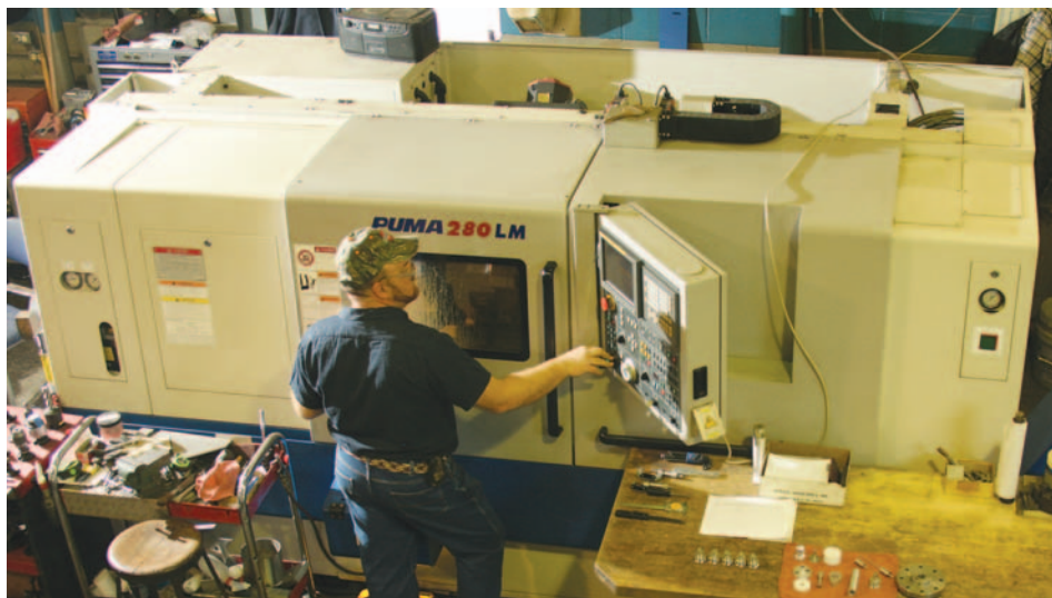
▲ Shickel Corp. still maintains a machine shop. The Puma mill/turning center, with its 16-in.-dia. by 40-in.-long capacity, is one of its recent investments to offer the latest in CNC machining technology.
