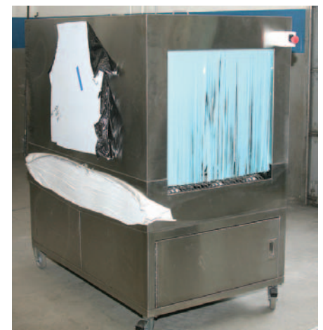
▲ An example of a stainless steel product that Shickel Corp. was contracted to fabricate is this sterilizing cabinet for an institutional laboratory. Employees fabricated the base and other components and then went to the customer's facility for on-site fit-up with the company's engineers. With tack welds holding the sterilizer components in place, a Shickel representative took it back to the shop for final assembly and finishing.
